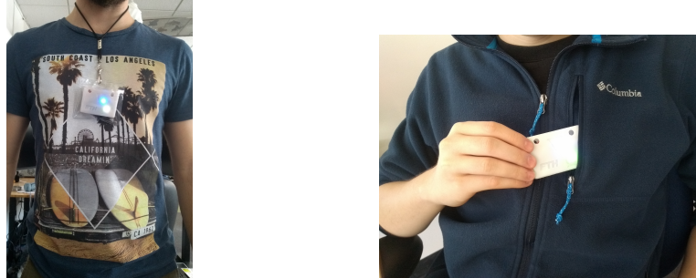
Figure 5.16: To find a suitable carrying mechanism, we test different approaches such as storing the node in the key pouch of trousers and using a pair of magnets to attach it to any kind of clothing. The two most popular methods are the use of a lanyard which is applicable to any kind of clothing (left) and the use of breast pockets found in shirts and jackets (right). Clearly visible in the picture on the left are the two status LEDs of the node: the upper one (blue) signals active neighbour discovery, while the lower one (green) indicates that the node is connected to an UWB network and performing rangings.
